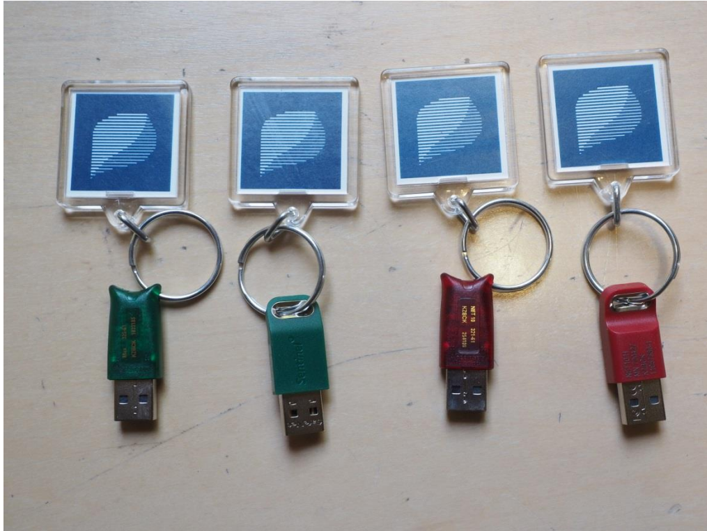
Figure 1: HL-Max key (green) and HL-Net key (red) are required for version 12 and higher. The first and the third key from the left have the old form factor. The other two keys have the new form factor. These two groups of keys have identical functionality.
