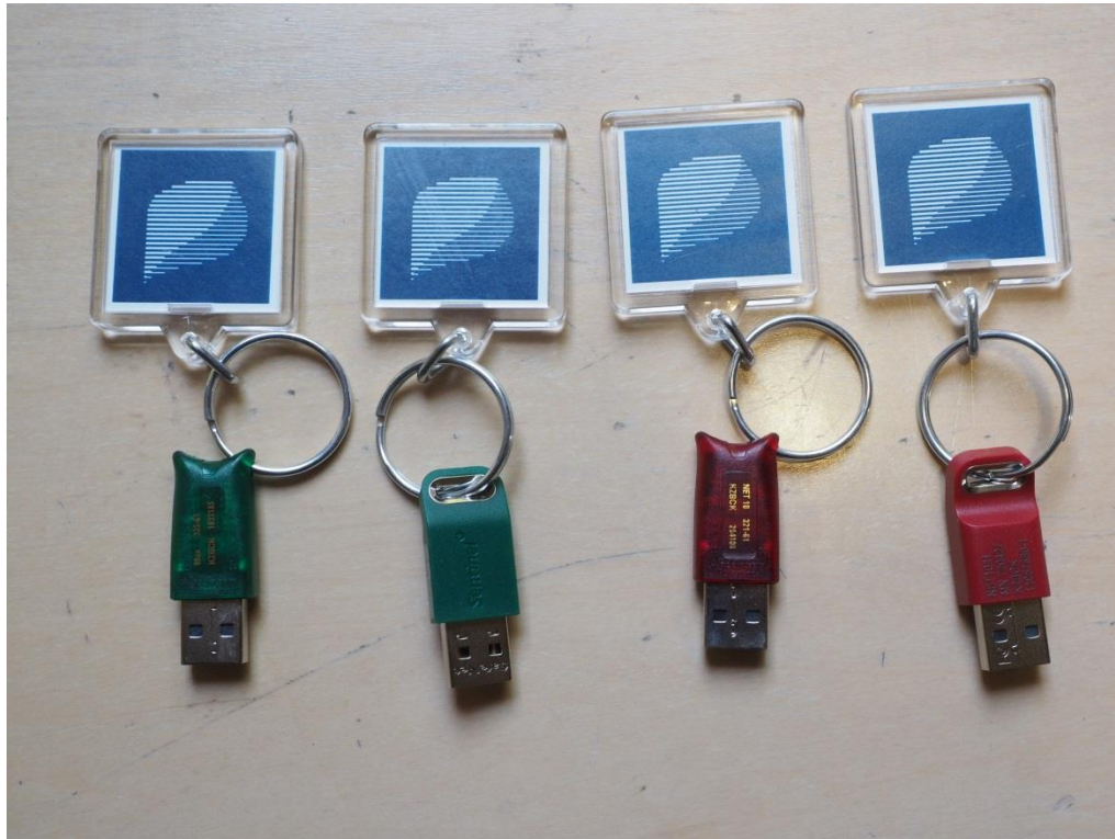
Figure 1: HL-Max key (green) and HL-Net key (red) are required for version 8 and higher. The first and the third key from the left have the old form factor. The other two keys have the new form factor. These two groups of keys have identical functionality.
