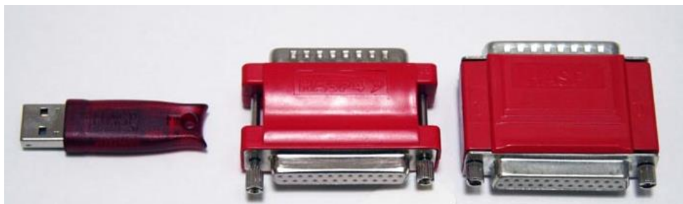
Figure 2: The long USB key and parallel-port keys are obsolete.
